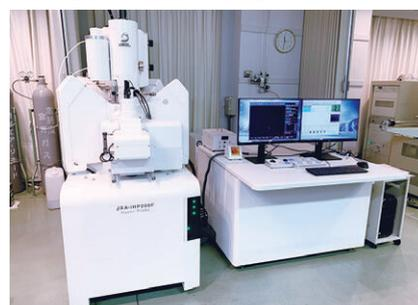
Electron probe micro analyzer (EPMA)
