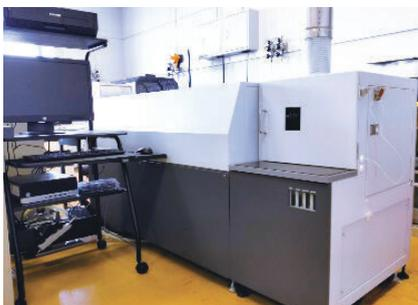
ICP optical emission spectrometer
