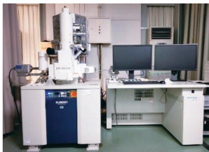
Field emission scanning electron microscope (FE-SEM)
