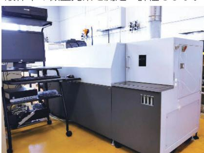
ICP optical emission spectrometer
