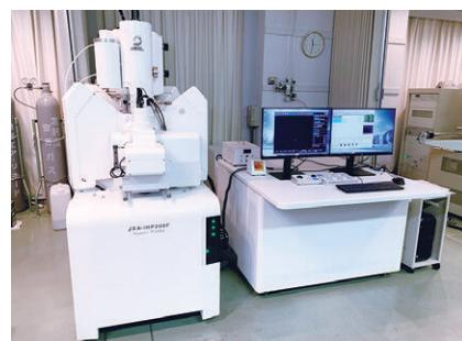
Electron probe micro analyzer(EPMA)
