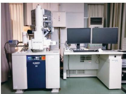
Field emission scanning electron microscope(FE-SEM)
